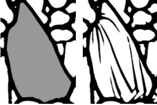
Figure 3. Left: segmentation of the calmes with the segmented tile in grey. Right: thresholding of the painted lines (and calmes)
