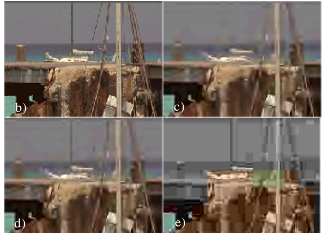
Figure 6. Sub-images (a) and (b) show the original image and a magnified sub-region. The sub-images (c), (d) and (e) presents the magnification of the compression result for JJ2000 (c), Kakadu (d) and JPEG-LS (e) for the subjective image quality evaluation.
