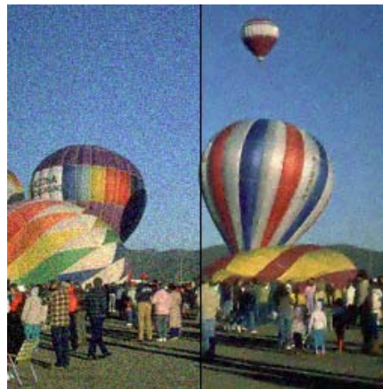
Figure 4. Demonstration of noise suppression produced by multiscale edgemap filtering (image is originally in color).
