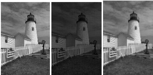
Figure 2. Example of a bilinear interpolation computed with convolution filters. Left: the original image (sub-sampled by a factor of 2 in the horizontal and the vertical direction). Center: one-color per pixel image according to the Bayer CFA. Right: image reconstructed with bilinear interpolation.
