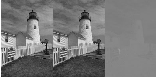
Figure 3. Decomposition of a color image (left) into luminance ( L=(R+G+B)/3 ) and chrominance ( \{R-L, G-L, B-L\} ).
