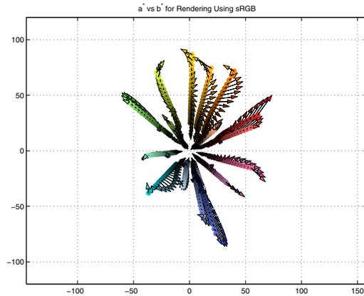
Figure 15. CIELAB hue constancy plots for sRGB when re-rendering output-referred images
