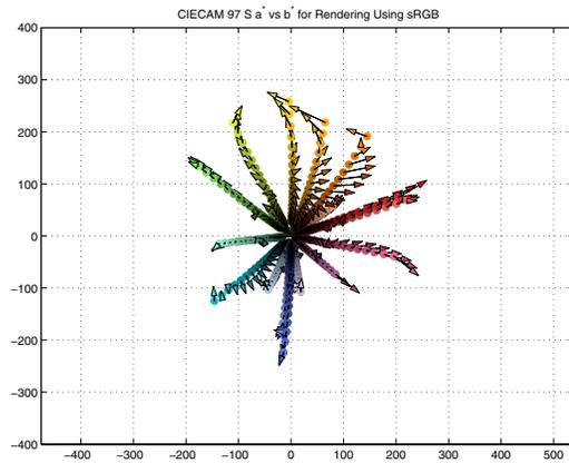
Figure 16. CIECAM97s hue constancy plots for sRGB when re-rendering output-referred images.
