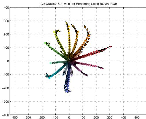
Figure 14. CIECAM97s hue constancy plots for ROMM RGB when re-rendering output-referred images.
