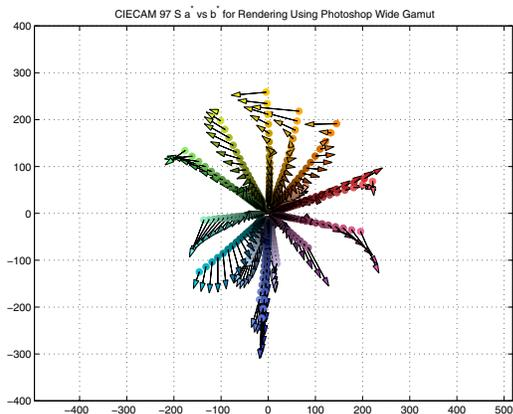
Figure 18. CIECAM97s hue constancy plots for Wide Gamut RGB when re-rendering output-referred images.
