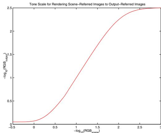
Figure 4. Tone scale used for rendering scene-referred to output-referred image
