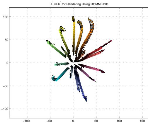
Figure 13. CIELAB hue constancy plots for ROMM RGB when re-rendering output-referred images.
