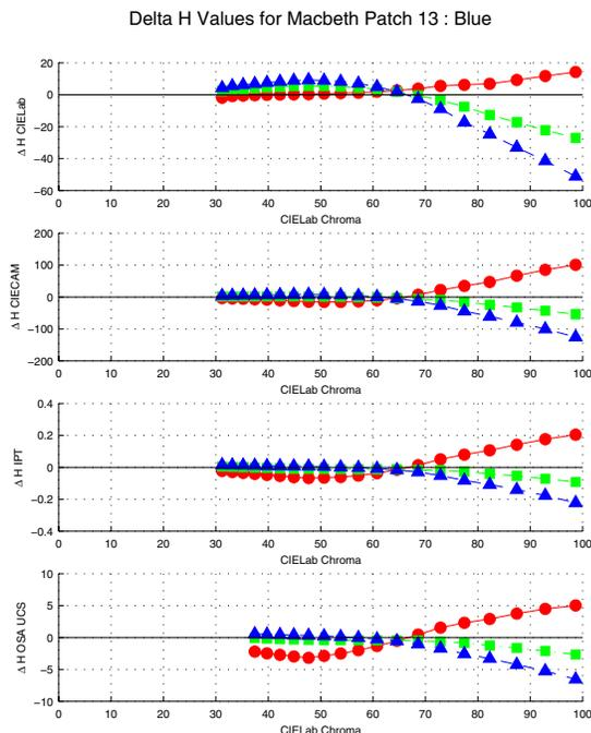
Figure 12. Hue shift plots for Macbeth blue patch highlight-to-shadow series for (top to bottom) CIELAB, CIECAM97s, IPT and OSA UCS (ROMM RGB: red circles, sRGB: green squares, Wide Gamut RGB: blue triangles).
