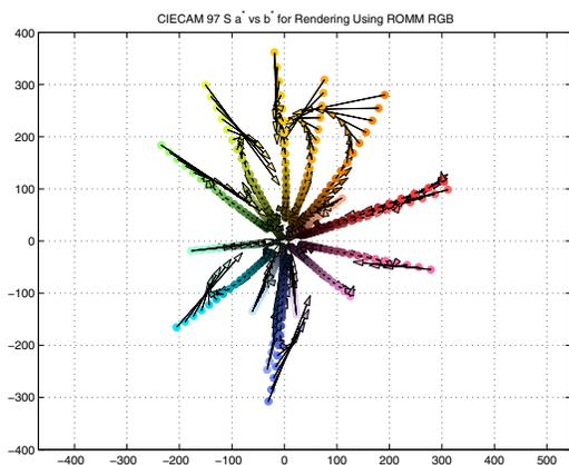
Figure 7. CIECAM97s hue constancy plots for ROMM RGB when rendering scene-referred images to output-referred images.
