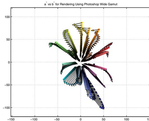
Figure 17. CIELAB hue constancy plots for Wide Gamut RGB when re-rendering output-referred images.
