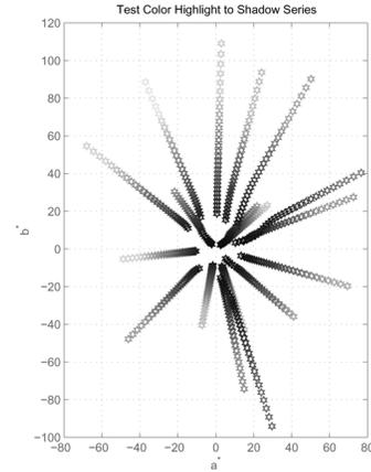
Figure 2. Highlight-to-shadow series for the test colors plotted in CIELAB  $b^*$  vs.  $a^*$ .
