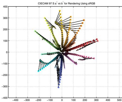
Figure 9. CIECAM97s hue constancy plots for sRGB when rendering scene-referred images to output-referred images.
