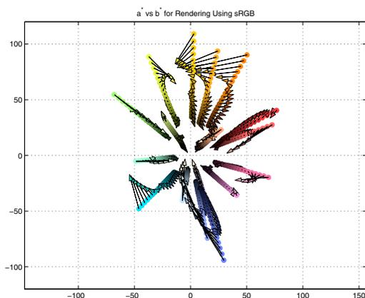
Figure 8. CIELAB hue constancy plots for sRGB when rendering scene-referred images to output-referred images.
