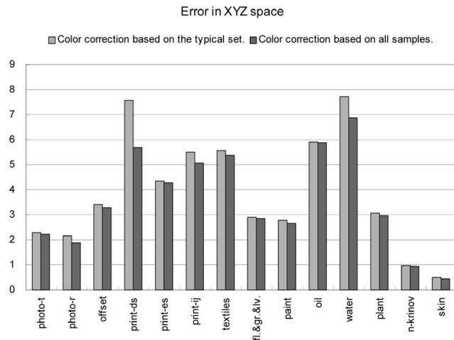
Figure 4. Residual rms errors after the linear color correction. (a) Photo (Reflection prints) (b) Electro-static printer (c) Textiles (d) Flowers, grasses & leaves
