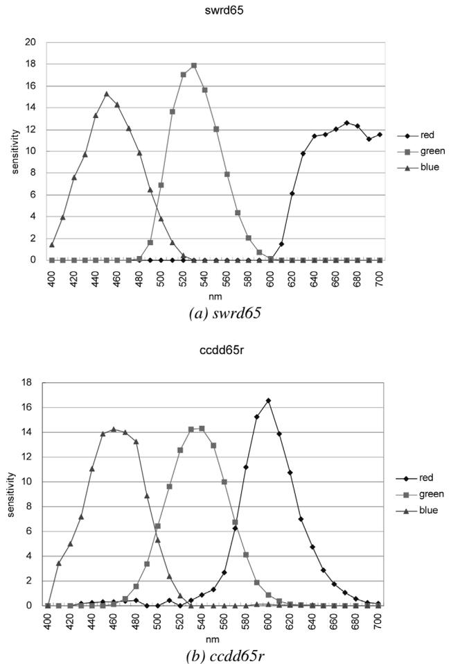
Figure 3. Spectral sensitivities of sensors used for the experiment.
