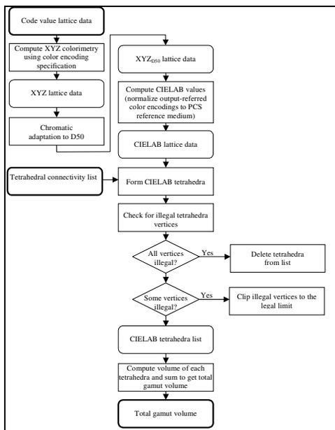
Figure A-1. Algorithm used to calculate the total gamut volumes of the CES (Metric 1).
