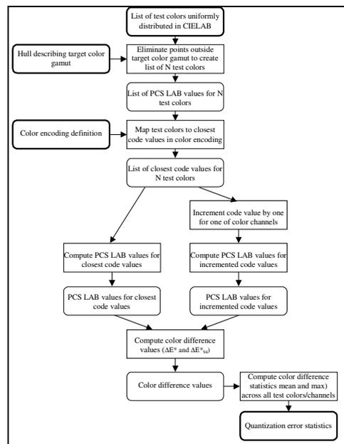
Figure A-4. Method used to calculate the quantization error statistics for the CES
