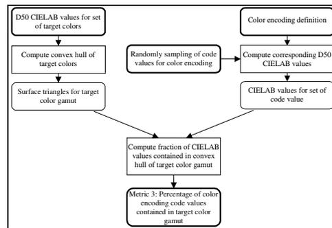
Figure A-3. Algorithm used to calculate the percentage of CES nodes contained used to encode the target color gamut (Metric 4).
