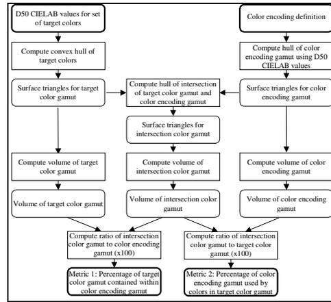
Figure A-2. Algorithm used to calculate the gamut volume intersections (Metrics 2 and 3).
