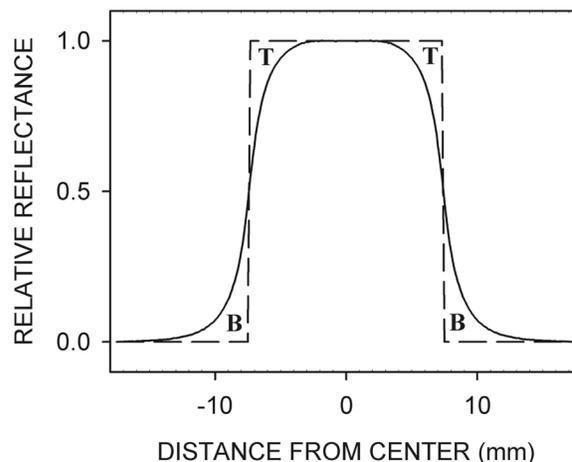
Figure 2. Narrow slit scan of a lighted area on a 0.1% TiO<sub>2</sub> loaded polystyrene exhibit (solid line) compared to an idealized scan of an opaque exhibit (dashed line).
