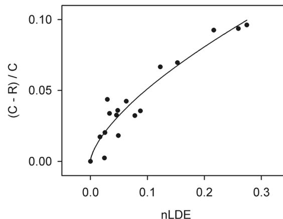
Figure 3. Measurements of 17 samples with the two channel detector system. Plot is the relative LDE versus the normalized center to ring values of the measurements. The solid line curve is a three parameter fit to the data.
