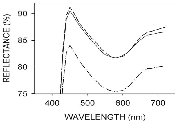
Figure 5. Corrected reflectance (upper dashed line) compared to 31mm illumination reflectance (solid line) and 4mm reflectance (lower dot-dashed line)
