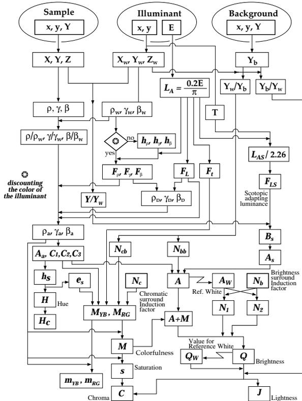
Figure 1. Flow diagram of Hunt appearance model.
