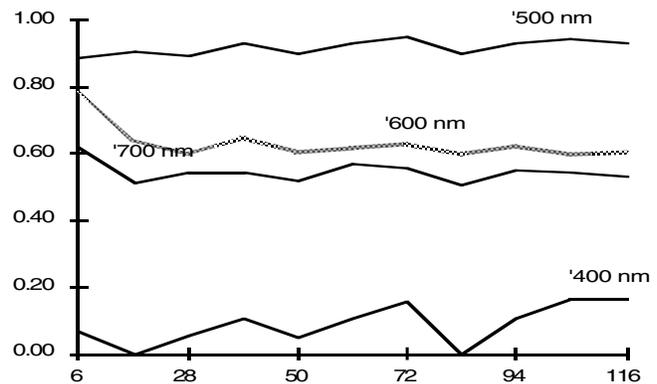
Figure 4. Relative sensitivity change across the CCD
