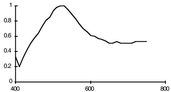
Figure 3. Average spectral sensitivity of the CCD
