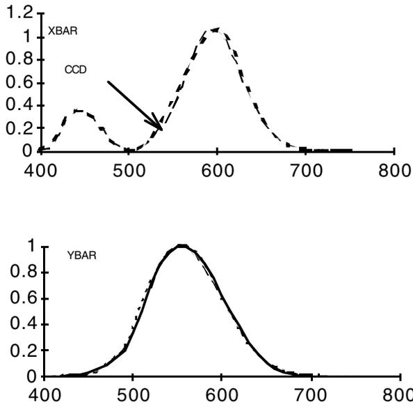
Figure 5.  $\bar{x}$  and  $\bar{y}$  sensitivities and CIE tristimulus functions
