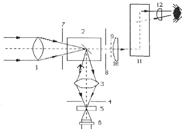
Figure 1. Single channel colorimeter input optics
