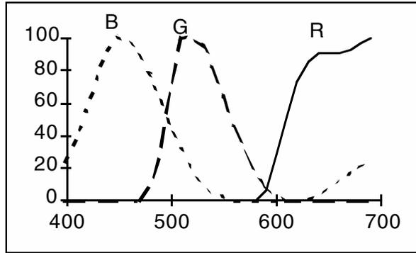
Figure 6 B, G, R spectral power distribution for LCD displays
