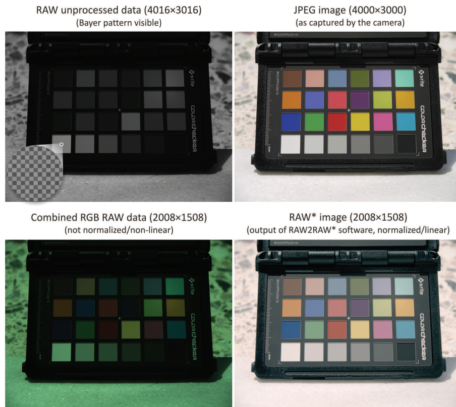
.Figure 14. Examples of RAW unprocessed B&W, JPEG image, combined RGB RAW data, and the RAW* output of the RAW2RAW* software.
