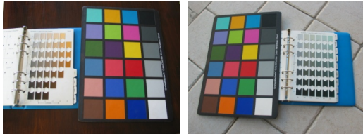
Figure 8. Example of image used to validate the color matching block
