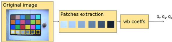
Figure 5. Color correction module using six neutral patches.
