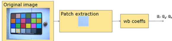
Figure 4. Color correction module using one neutral patch.
