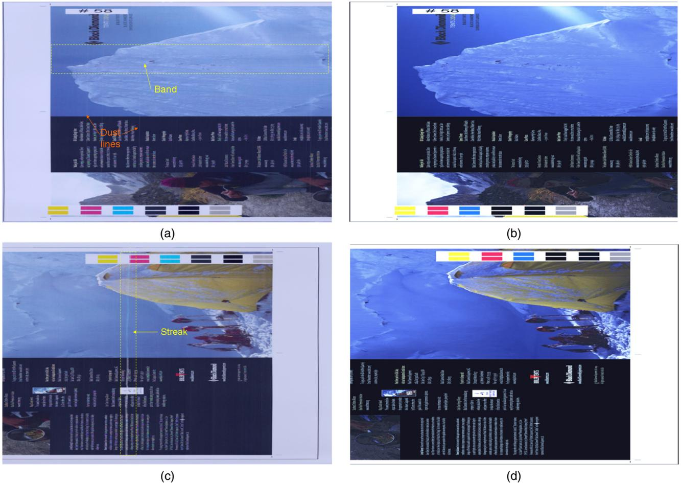
**Figure 2.** (a) shows a scanned document after registration which contains a band. In addition, the scanned image contains some vertical dust lines that come from the scanning process. (b) shows a digital reference of (a). (c) shows a scanned document which contains a streak and (d) shows the corresponding digital reference.
