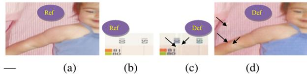
**Figure 1.** Close up on originals (a: Ref, left) and scans (d: Def, right) of two images after color and position registration. Arrows point to faint scratch artifacts on Def images. The most prominent local differences are contrast and detail loss in Def. This type of scratch artifacts is so faint that you may need to look on an enlarged digital version to see the artifacts.
