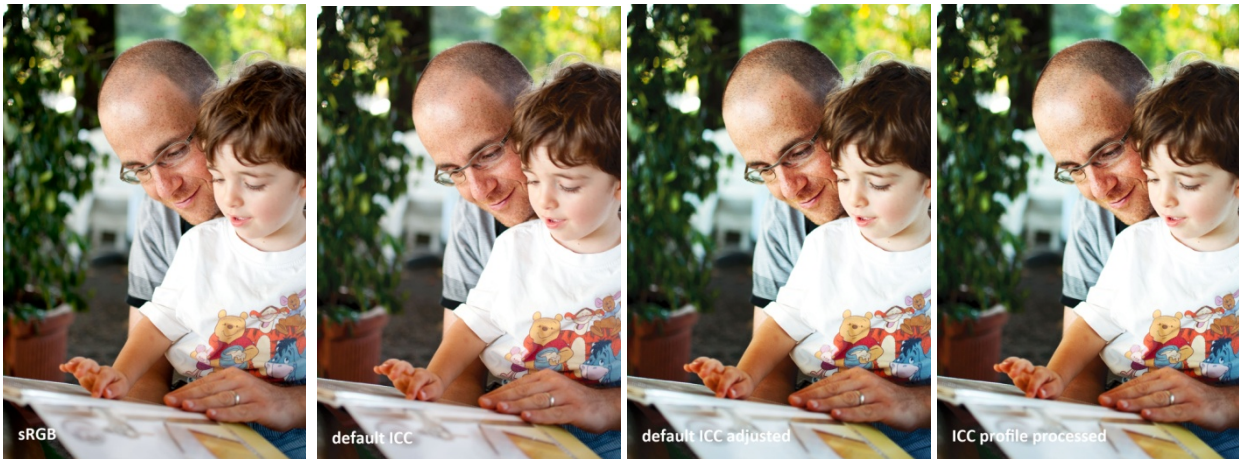
Figure 5. From left to right (sRGB previews): original unadjusted image in sRGB color space, unadjusted image converted to a reference printer ICC profile, adjusted image in reference printer profile space, unadjusted original image (left most above) converted to newly processed ICC profile.
