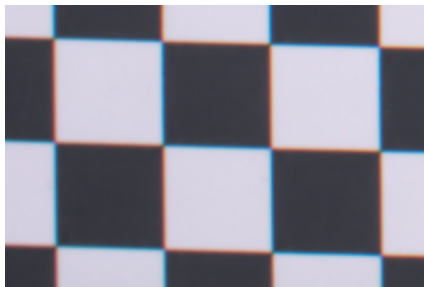
Figure 1. Chromatic aberrations on the bottom left corner of the image of a checkerboard pattern.
