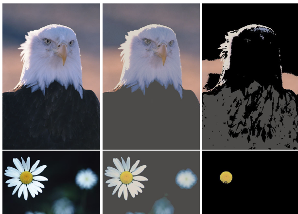
Figure 4: The original images are listed in the left column, the gamut mapped ones are in the middle and the results from the global method are shown on the right. For the first row, the global saliency detection generally tells where the artifacts lie. However, in the next row, the heart of flower stands out of both original and reproduced image. The global thresholding is no longer sufficient to detect the artifacts.
