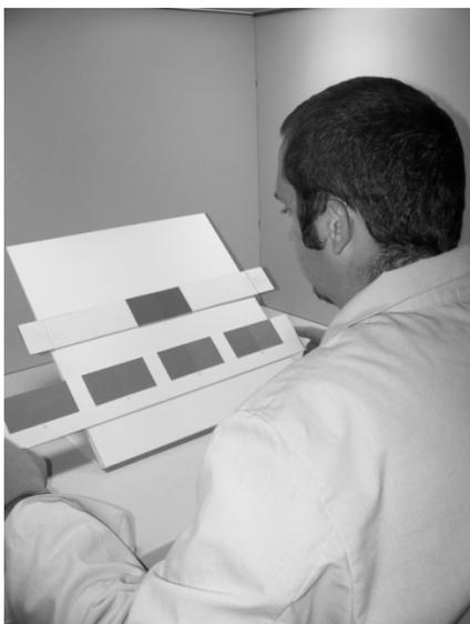
**Figure 2.** Sample stand, viewing and illumination arrangements used in the NCSU-2 dataset employing a perceptually linear gray scale.
