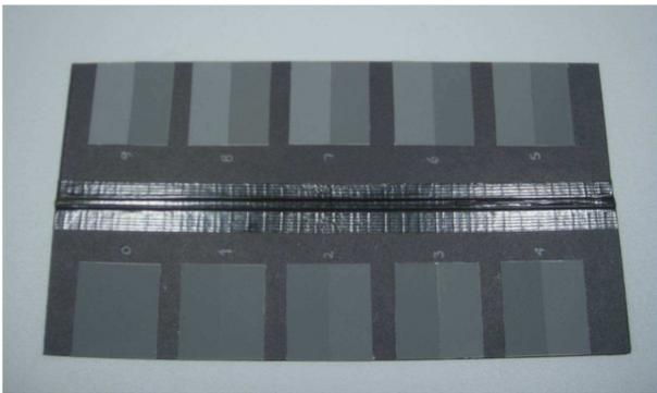
Figure 5. Prototype perceptually linear gray scale constructed for comparison against the AATCC gray scale for color change.
