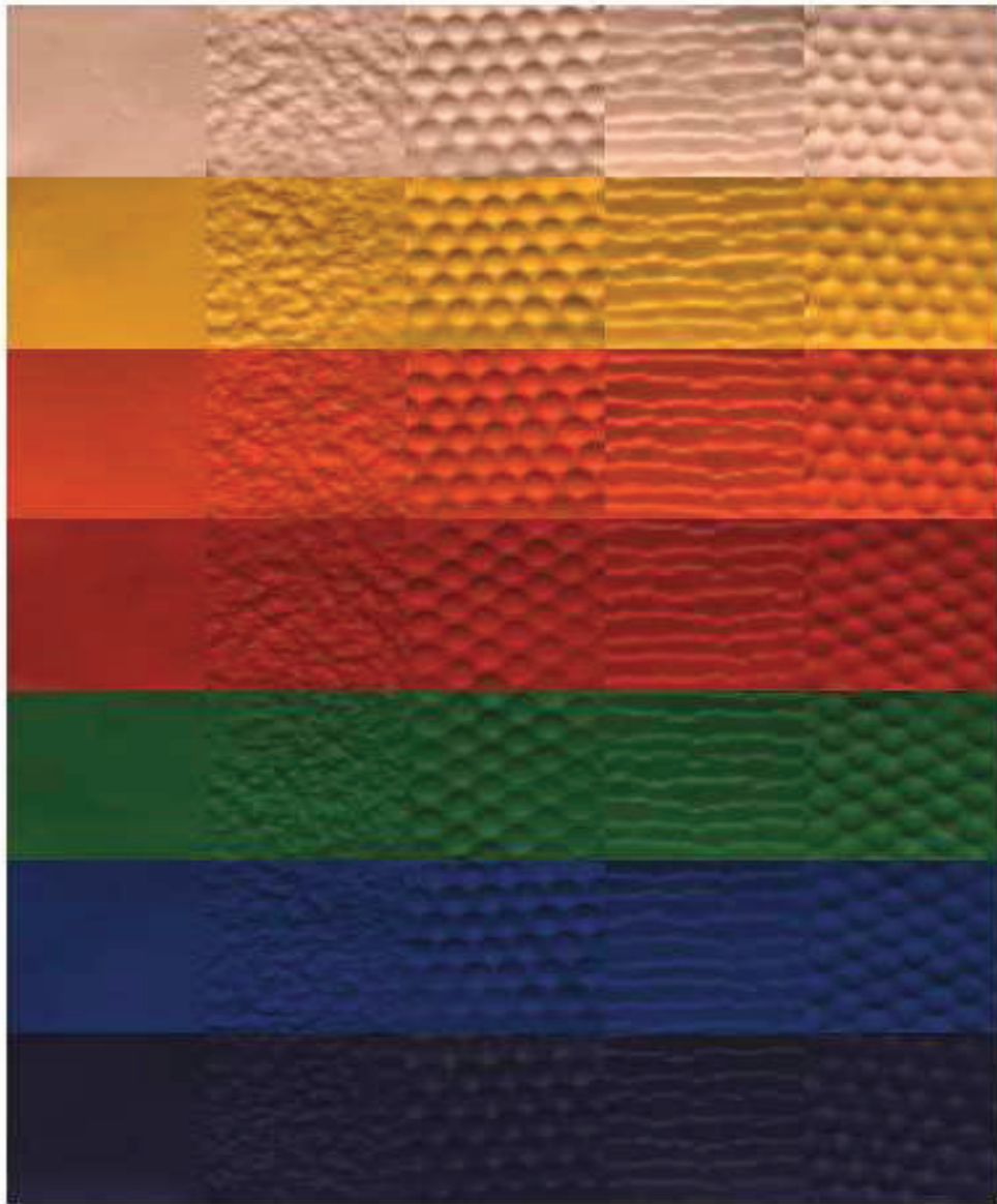
Figure 3: The seven textured colored sample set. The samples are organized in seven sets of five samples of the same color (pale pink, yellow, orange, red, green, blue and purple), having each one the same color but different texture (flat, random, convex hemispheres, irregular in one direction and concave hemispheres).
