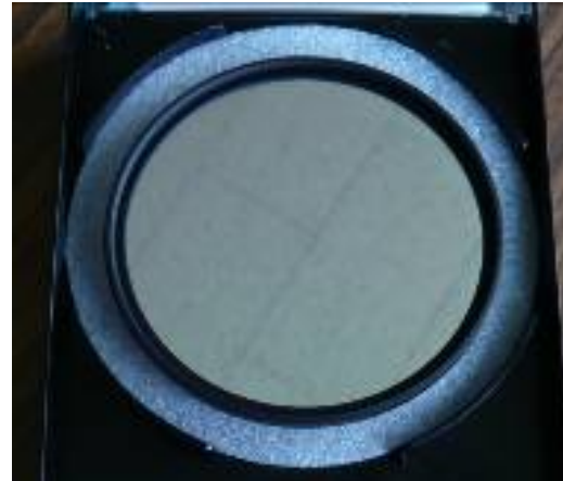
Figure 4. Developed optical filter. The optical filter was made of multi-layer thin film to realize the theoretical spectral transmittance shown in Fig. 3.
