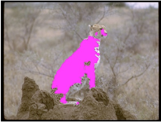
Figure 5. Final segmentation of the original image is shown in Figures 1 and 2. Pixels in pink are considered to belong to the desired region.
