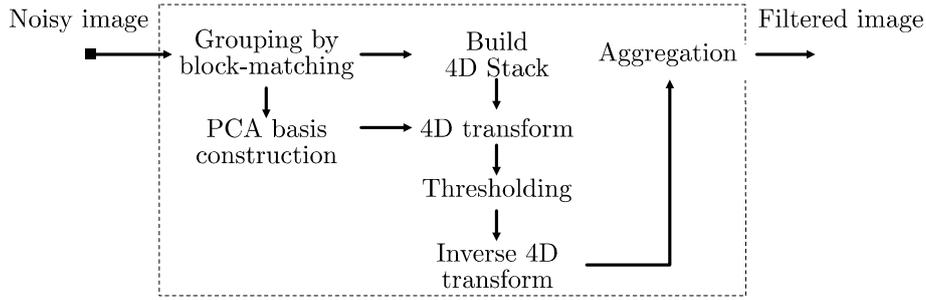
Figure 1. Flowchart of the proposed MSPCA-BM3D algorithm.
