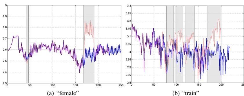
Figure 15. The fractal dimension as a function of time (blue-original, red-received / degraded) for the "female" and "train" video seq.
