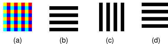
Figure 3. A colored pattern and its components (a) RGB channels, (b) red, (c) green, and (d) blue channel. The square structure which is clearly visible in the color pattern is not present in any of the channels.
