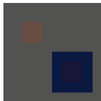
Figure 5. Example of images with same CIELAB units between two pairs but different visual perception
