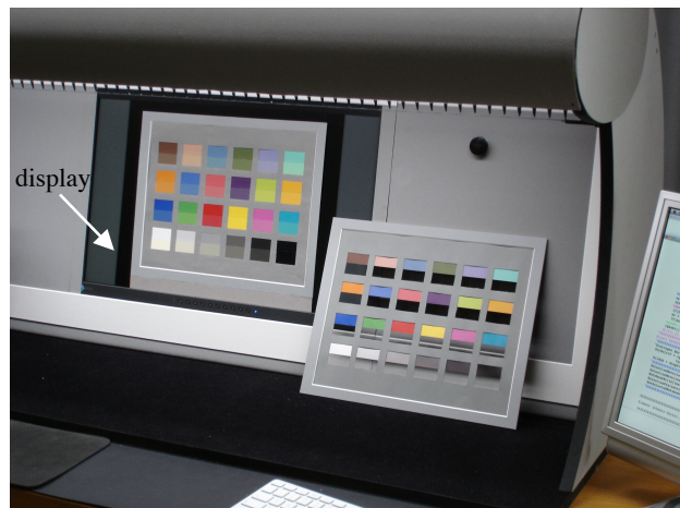
Figure 2. Laboratory model of a softproofing station equipped with 24" LCD-Display and a mask in front, providing the colours of a color checker. A second colour checker mask is shown in front.
