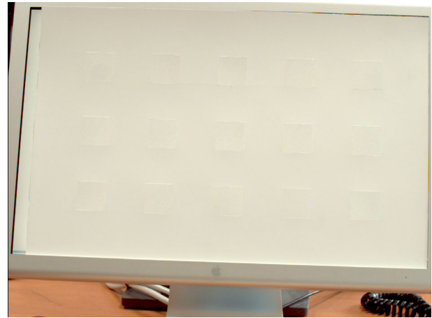
Figure 10. Acquired image of the calibrated monitor with the calibration mask applied; the brightness of the monitor cut-out areas perfectly match with their surrounding brightness values. Therefore, the mask can hardly be identified.
