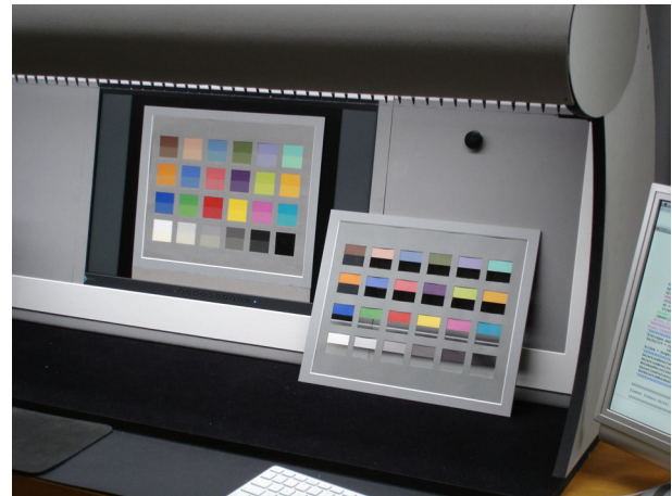
Figure 1. The softproofing system with its built-in illumination at the top side makes a critical side-by-side comparison between objects and their reproduction on the monitor feasible.
