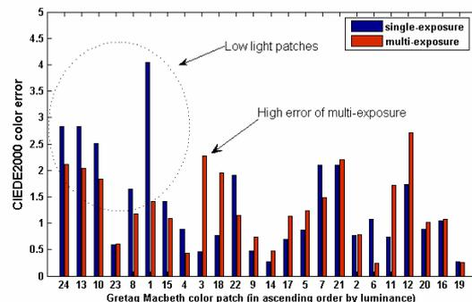
Figure 11. CIEDE2000 colour error values for paper p5 ordered in ascending order by measured luminance of patches
