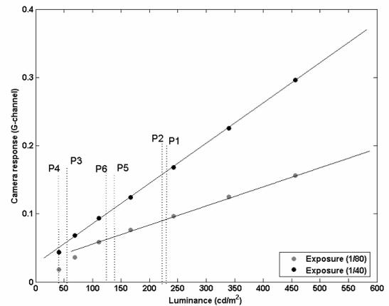
**Figure 5.** Camera responses for exposures 1/80s and 1/40s in scale 0 – 600  $\text{cd/m}^2$
