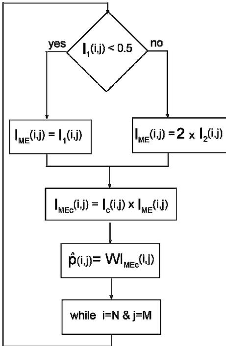
**Figure 3.** Flow chart for spectra,  $\hat{p}$ , reconstruction in pixel position,  $(i,j)$ , where  $I_1$  is long-exposure image (1/40s) and  $I_2$  is short-exposure image (1/80s),  $I_{ME}$  is multi-exposure image,  $I_C$  is pixel-wise correction matrix,  $I_{MEC}$  is corrected multi-exposure image and  $W$  is transformation matrix solved by the method proposed by Shen and Xin [13]
