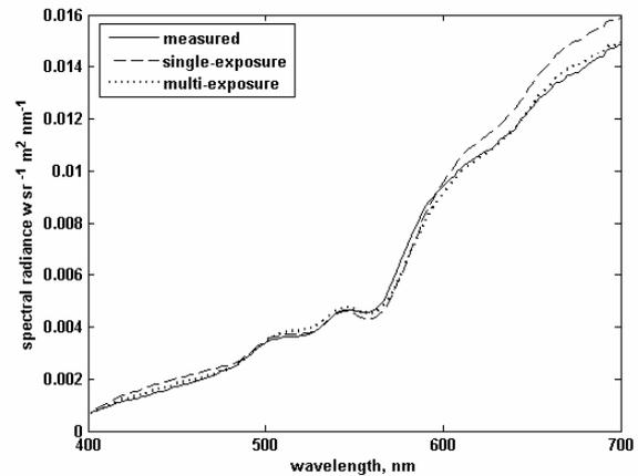
Figure 9. Spectral radiances for dark brown patch (patch number 1) in Gretag Macbeth CC test target printed on paper P5
