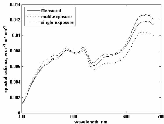
Figure 12. Spectral radiances for patch number 3 printed on paper P3
