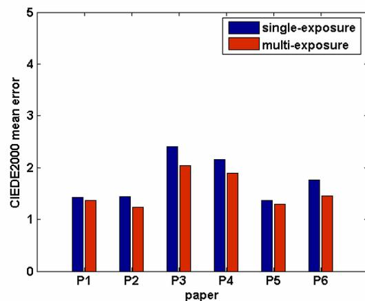
**Figure 6. CIEDE2000 mean colour error values of different paper grades using single-exposure and multi-exposure methods for testing samples**
