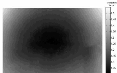
**Figure 2.** Intensity image of correction factor matrix for green channel in our measurement environment
