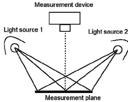
**Figure 1.** The measurement environment includes two halogen lamps (3097 K), measurement plane for samples and measurement device holder perpendicular to the measurement plane
