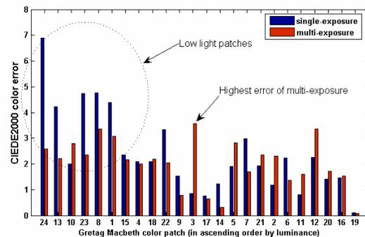
Figure 10. CIEDE2000 colour error values for paper p3 ordered in ascending order by measured luminance of patches
