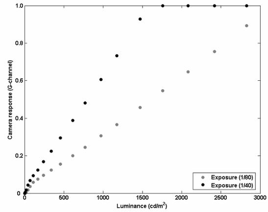
**Figure 4.** Camera responses for exposures 1/80s and 1/40s in scale 0 – 3000  $\text{cd/m}^2$
