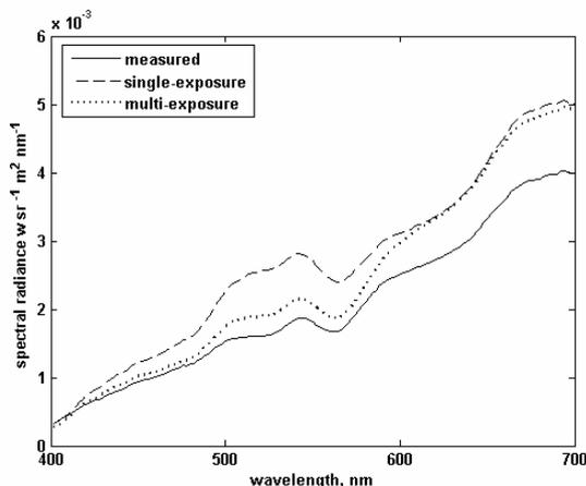
Figure 8. Spectral radiances for dark neutral patch (patch number 24) in Gretag Macbeth CC test target printed on paper P3
