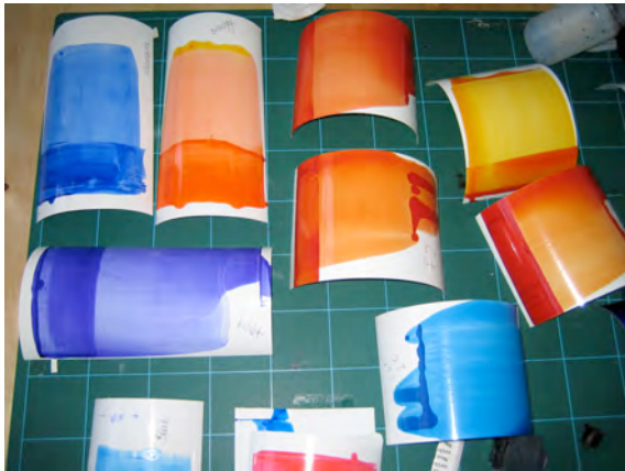
Figure 1. Sheets of semi gloss paper were initially coated with the original Vivera CMYKcLm inks using a K-Bar, allowed to dry and were then measured.
