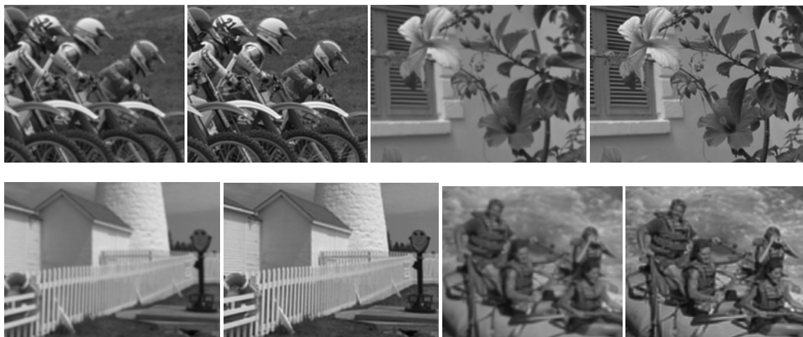
Figure 5. This shows results for the intermediate luminance approximation from scalar-valued color sensor data. The first image of each scene pair shows the Gaussian filtered Bayer image, and the second shows the deburred result taken for a high spatial resolution luminance image.
