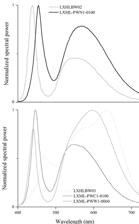
Figure 2 - Normalized spectral power distribution of the 5 white LEDs used (Luxeon, Philips Lumileds Lighting Company, USA).
