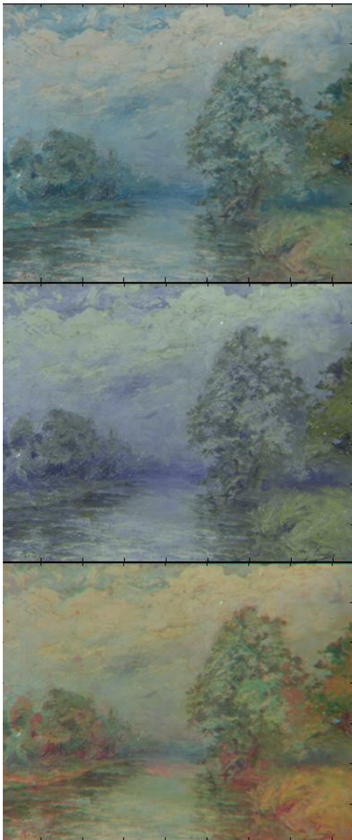
Figure 7. Color thumbnails of one artistic painting under D_{65} (upper picture) and under two metamers of D_{65} (middle and lower picture).
