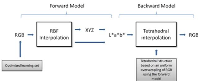
**Figure 2.** Overview of the colour characterization model of the display
