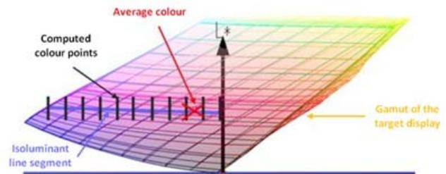
**Figure 3.** Computation of the different background colours based on a chromatic path derived from the average colour of the displayed image
