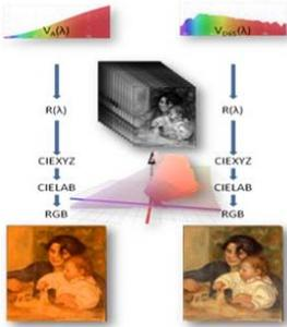
**Figure 1.** Colour workflow, from a multispectral image to a reconstructed colour image
