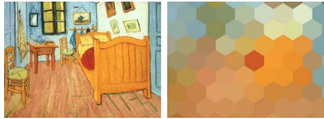
Figure 5. Coarse segmentation (right) of a colour image computed from multispectral data (left)
