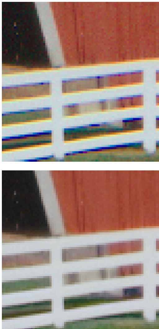
Figure 8. Cropped 200 ppi six color scans without FCCT (top), and with FCCT (bottom).
