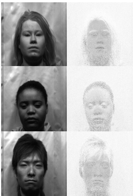
Fig. 9. The images shown on the left are 900 nm channel images. On the right the ratio images 980 nm/900 nm are shown. The spectral imaging was done on real faces.
