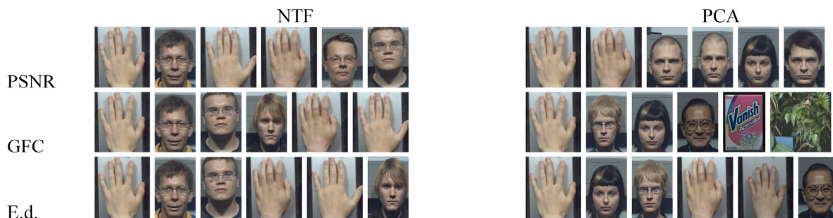
Figure 11. Ordered output for spectral images in the case of NTF and PCA features uses. The similarity measures used, row by row from top to bottom are: PSNR, GFC and Euclidian distance.
