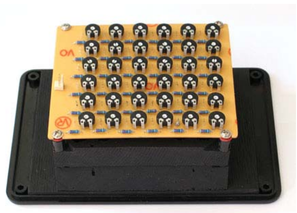
Figure 3. View of the assembled components after rear cowling removed with the filter array faceplate at bottom then the mixing chamber and PCB uppermost.
