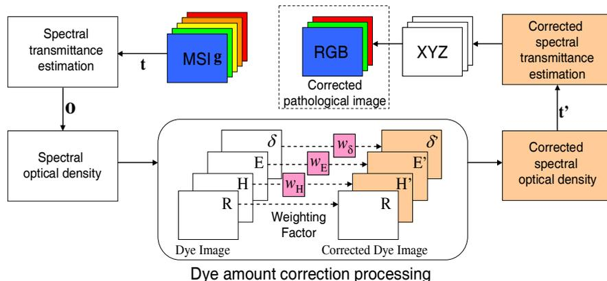
Figure 2. The process of the modified color correction method in RBC areas based on multispectral imaging technique and Beer-Lambert law.
