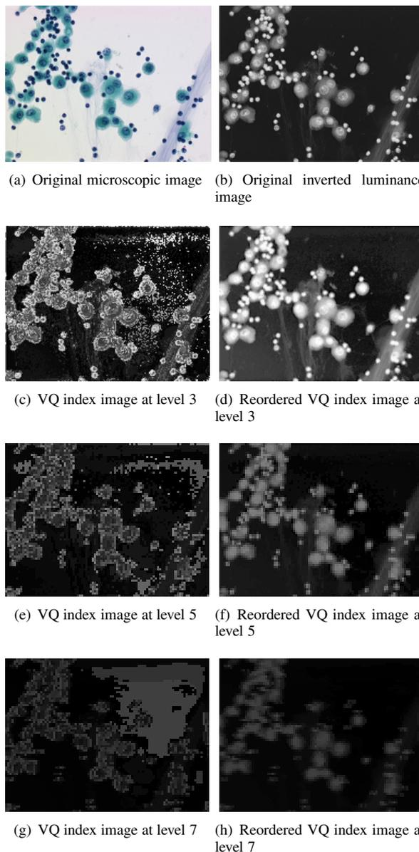
**Figure 6.** Obtained rough VQ index images (c,e,g) and reordered VQ images (d,f,h) at the three different levels of the pyramid. Image (b) represents the initial inverted luminance image of the original image (a)
