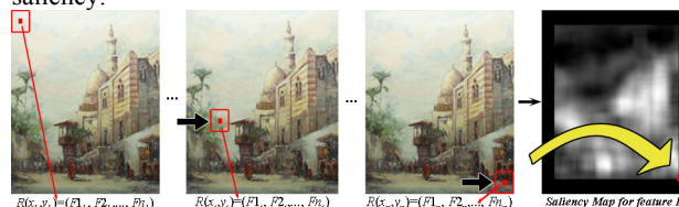
Figure 2. General principle of feature map computation: for each pixel position, a neighbour is defined, the feature is computed using the neighbour influence, leading to one pixel value in the final feature map (see on the right)
