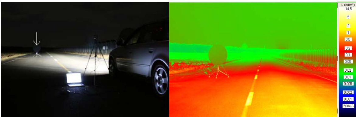
Figure 2. A mesopic road lighting scene with a circular visual target (left picture, below the white arrow). The scene was measured at night by a video-photometer with 4 filters (X, Y, Z, and V). The target appeared at 5.4° left to the optical axis and its diameter was 2.3°. Right picture: photopic luminance distribution next to the target.
