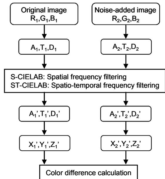
Fig. 1 Basic flow for calculation of color difference common to S-CIELAB and ST-CIELAB.
