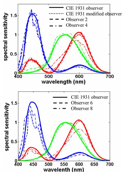
Figure 1. Colour matching functions for different real observers and the CIE 1931 observer at the G94 system.
