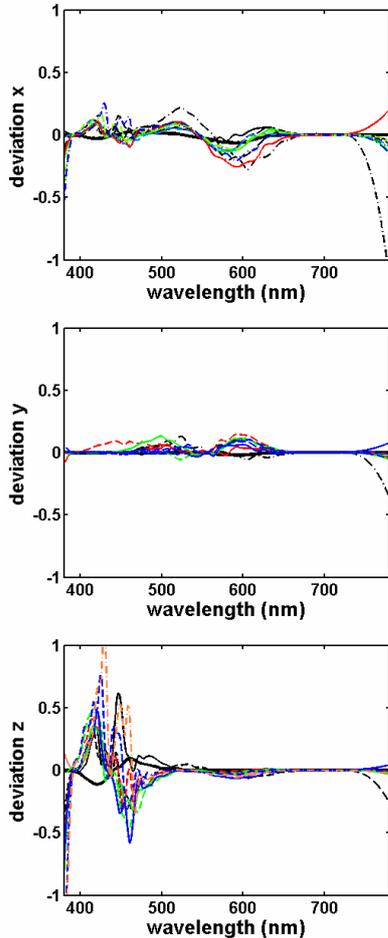
Figure 2. Deviation functions of the 10 real observers and the first deviation functions defined by the CIE (CIE 80:1989) with the CIE 1931 standard observer (black solid line).
