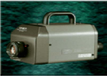
Figure 2. The Minolta CS1000 tele-spectroradiometer, used to measure the office lighting in terms of SPD
