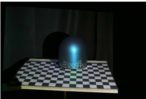
Figure 4. Environment mapping is added to simulate the appearance of a clear coat. Here, the metallic blue simulation shown in Figure 3 is given a glossy finish.
