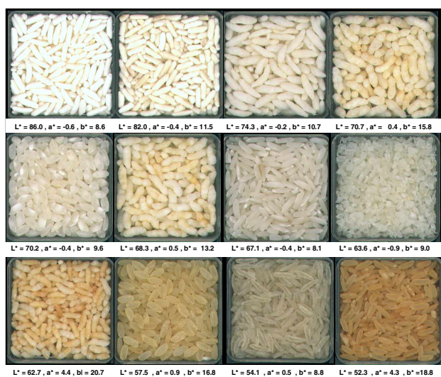
Figure 2. FBS images of a selection of calibration and validation samples used for the determination of the bulk colour.
