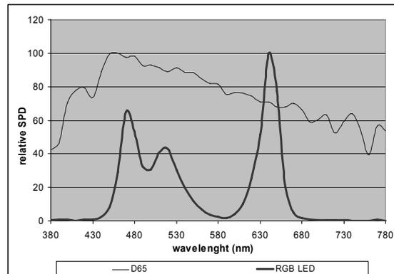
**Figure 6.** Relative spectral power distributions of D65 (thin curve) and our test white RGB LED light source (thick curve).
