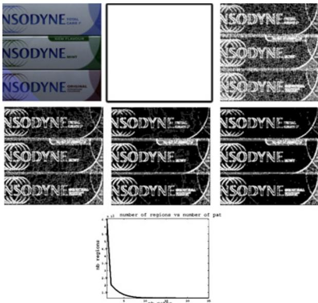
**Figure 4.** From left to right and top to bottom: The original image and the segmentations after 1 (all white since the first step is to label all pixels differently), 2, 5, 10 and 15 paths respectively. The curve on the 3rd row shows the speed of convergence for this particular image.
