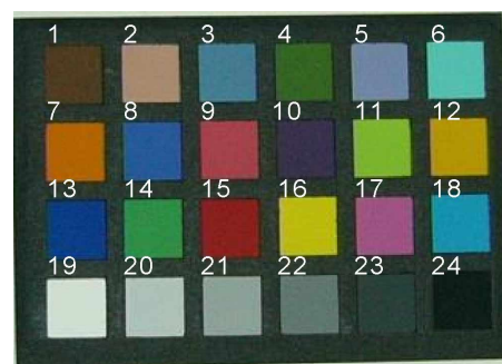
Fig. 4 Macbeth Color Checker used for spectral reflectance estimation.
