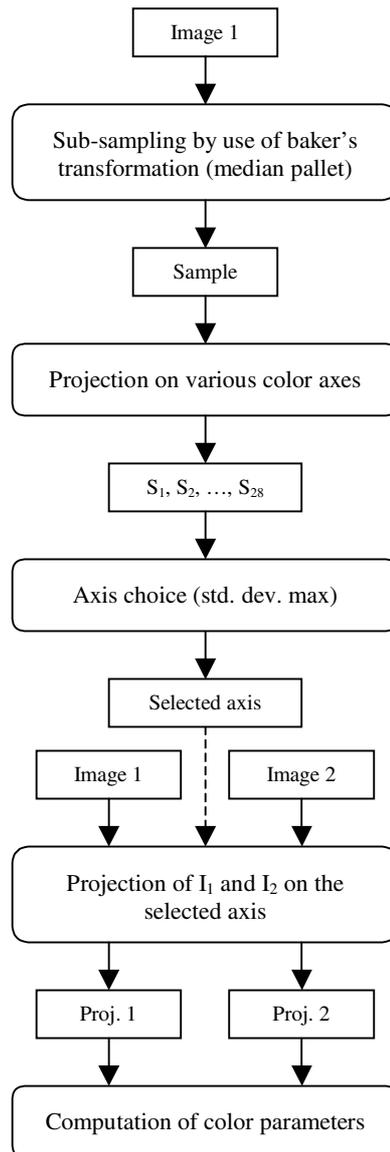
Figure 6. Sub-process for computation of color parameters.
