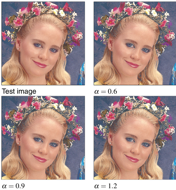
Figure 12. The result for sharpening within the gamut (a) for different values of \alpha , with \sigma = 1 . The original image is smoothed with inverse unsharp masking with \alpha_{inverse} = 0.6 . masking.
